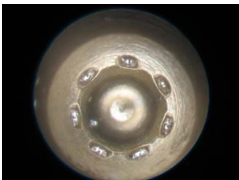
Figure 5a. Boroscope image of the interior of a 7-orifice nozzle coated with EN to a final orifice size of 75 \mu\text{m} .
