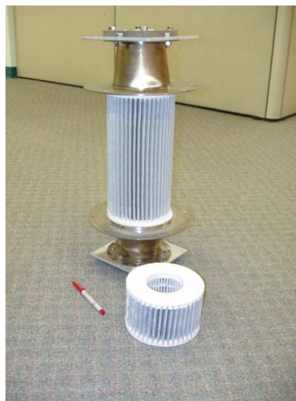
Figure 14. Full-scale 6-in.-diam × 12-in.-long long round pleated filter ready for canning and truck testing (first prototype shown at bottom of figure).
