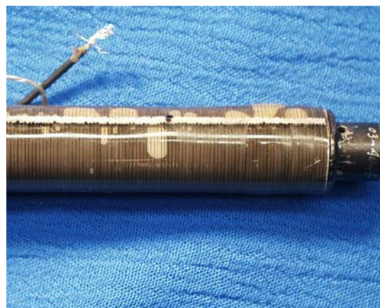
Figure 4. Large KCI actuators after failure in high-pressure hydrogen tests. Optical microscopy reveals the most obvious change after testing, which is the formation of the delamination regions or bubbles beneath the outer epoxy layer on the actuators.
