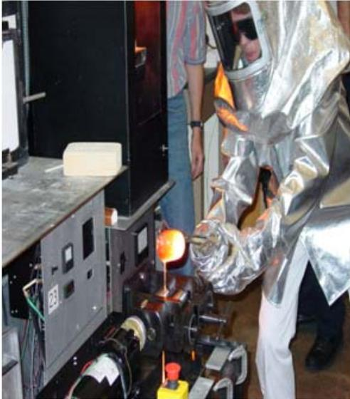
**Figure 2. Glass ceramic sheet formation by pouring molten glass on a roller.** The sheets made by this process were provided to TRS Technologies for incorporation into a multilayer capacitor.
