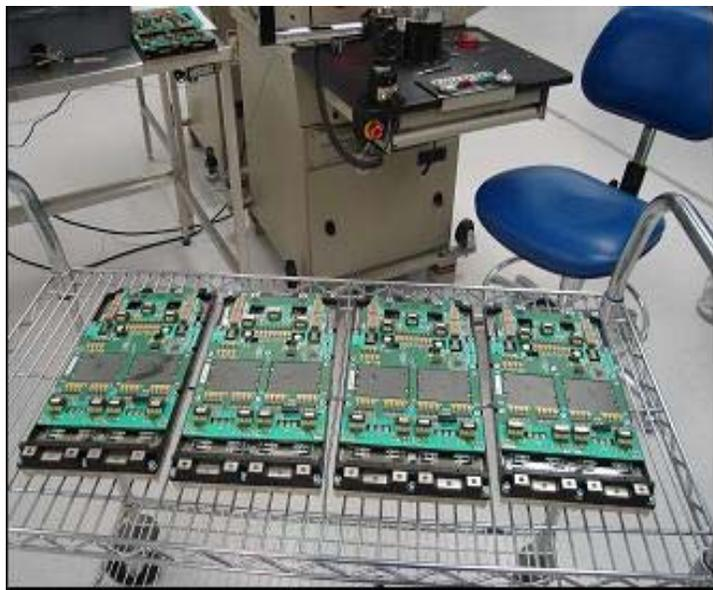
**Figure 7. Completed ORNL Beta power modules.**
