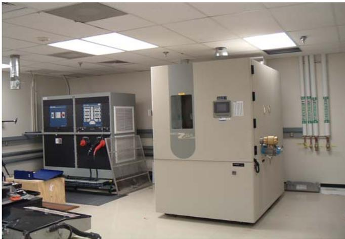
**Figure 1. Environmental Chamber and ABC100—125-kW bi-directional power supply**
