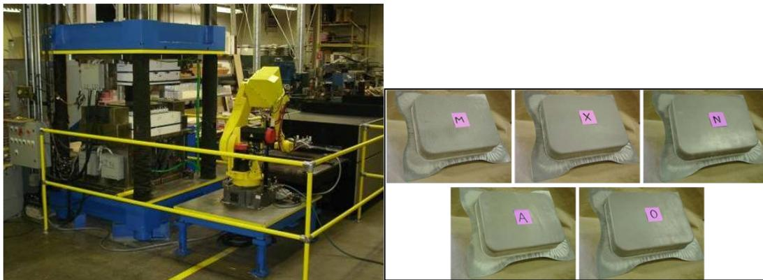
Figure 1. Warm forming cell capable of five jobs per minute and pans stamped at 350°C from five different magnesium alloys.
