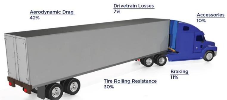
Figure 23. Power Use Diagram for a Class 8 Tractor-Trailer Shows a typical percentage distribution of the mechanical power losses for a long-haul usage (varies based on the particular drive cycle)
