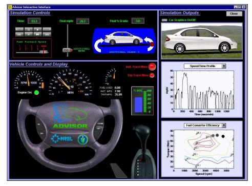
ADVISOR can predict vehicle performance, energy consumption, emissions output, control strategy function, and average component efficiencies over multiple driving cycles and test procedures.
