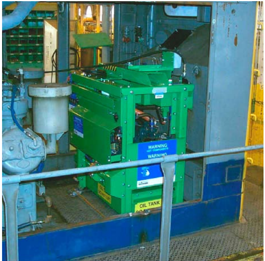
K9® APU installed on a locomotive
