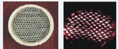
*The new ceramic fiber particulate trap employs an efficient, microwave heating cycle to regenerate itself. A pleated design (below) will be useful for high-volume exhaust streams.*
