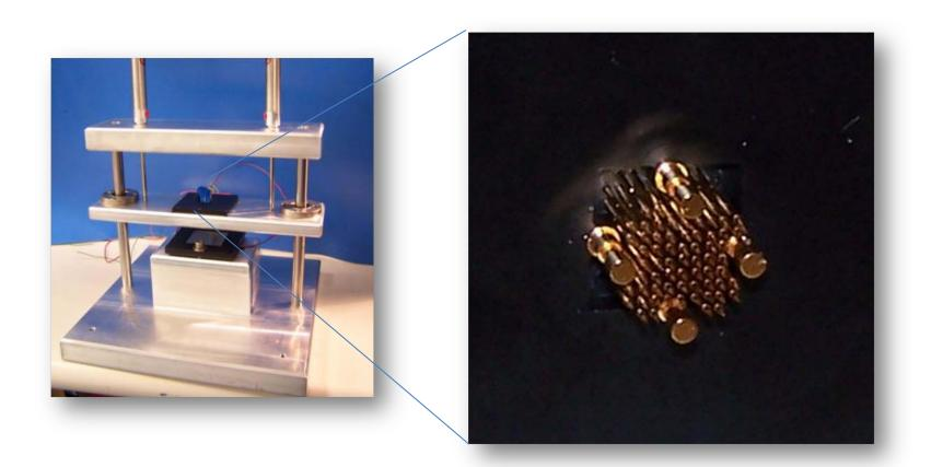
60 voltage probes and 4 thermocouples
