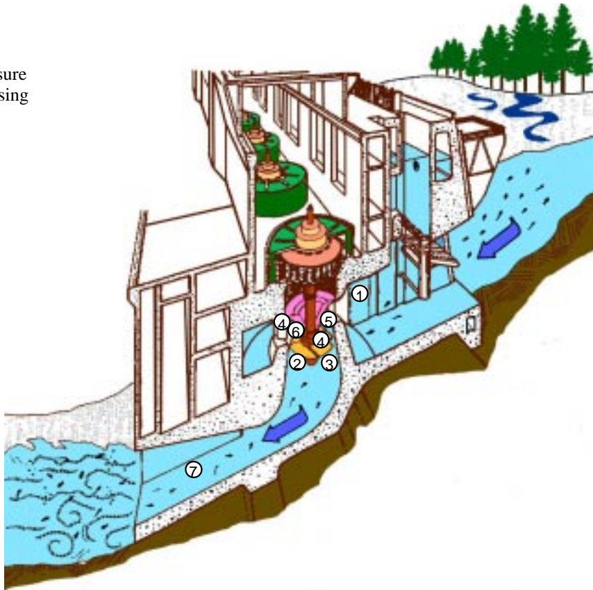
Figure 2. Schematic diagram showing locations within a turbine system where fish injury mechanisms are believed to occur. (Modified from: Čada et al. 1997)
