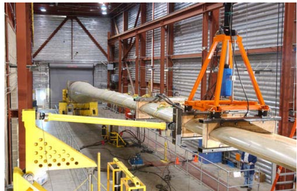
Figure 6. Blade undergoing structural testing
